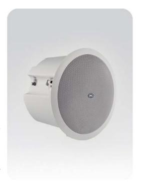
The built-in 8" speaker driver is designed of wide frequency response 60-2kHz, the multiple power taps 3.8W, 7.5W, 15W, 30W & 60W are helpful for different applications varies from room size and ambient noise surroundings. The metal grille, ABS baffle and ABS back cover are painted in attractive RAL9016 white color. Its flush mount type makes the easy and secure installation.
